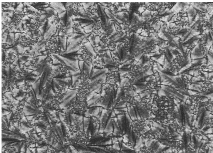
Figure 4; Focal-conic fan shape texture with equidistant lines of poly(6-8) with DP=24 obtained at 69 °C upon cooling from the isotropic phase.
